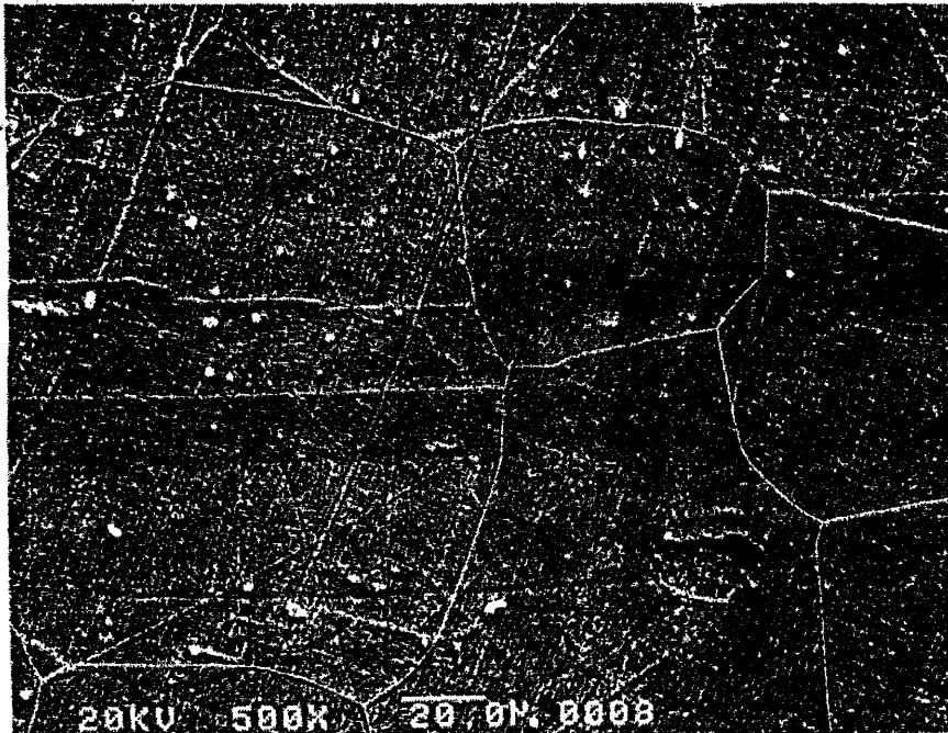
Fig. 3.25(d). Surface appearance of irradiated N10 (x500) after exposed to Moc-EPR. The lighter tone region as seen in the above lower-magnification micrographs is shown here. [EPR ratio: 0.0% (first peak) and 70.1% (second peak)]
