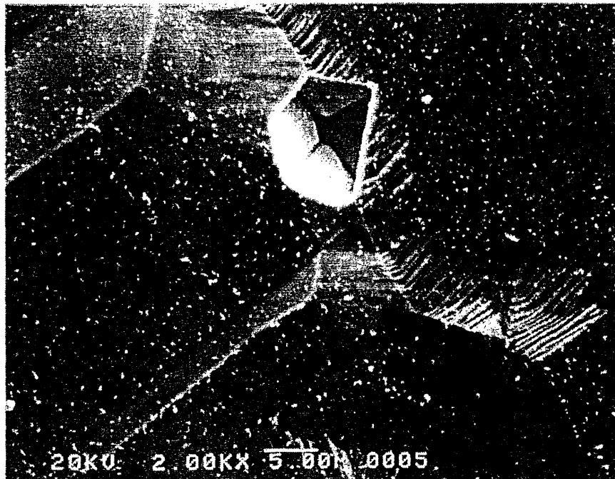
Fig. 3.23(d). Surface appearance of irradiated N6 (x2000) after exposed to Moc-EPR. [EPR ratio: 0.112%]
